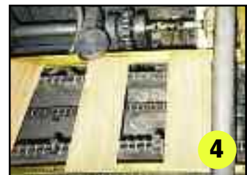
4 The graphite cores have been glued into place in the upper row of slats. Soon, the upper and lower slats will be joined together and cut into ten pencils.
