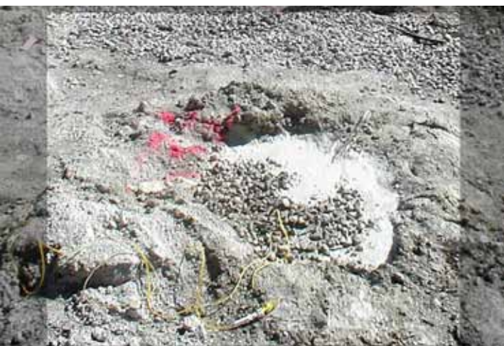
In this file photo, the highlighted area shows a drill hole filled with explosives and fuel at the Magruder quarry location. The blasting cap and lines are visible as well. Scores of these lined the rock face in order to blow a section away in a massive rippled explosion. This blasting, the city of Osage Beach says, is responsible for damage to their sewage facility.
