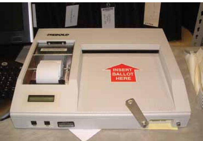
To use the machines, voters slide their ballots into the slot on the right and after those ballots are "read," voters are told whether they were counted or if a mistake was made and a new ballot is required.
