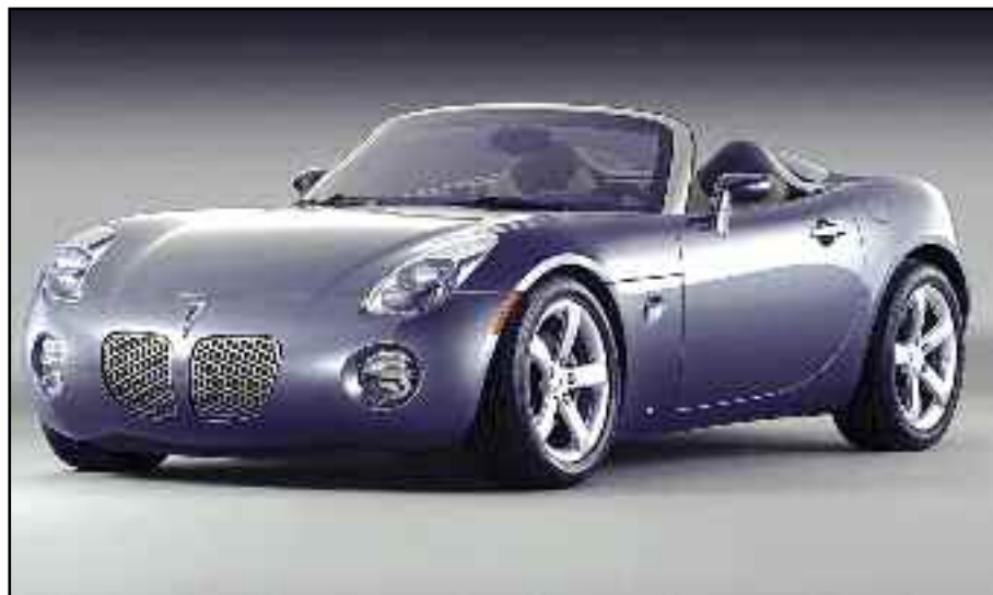
2006 Solstice debuts as the first two-seat convertible at Pontiac since 1940. The rear-wheel-drive Solstice is an eye-catching roadster with a wide track and 170-horsepower, 2.4-liter, four-cylinder Ecotec engine.
