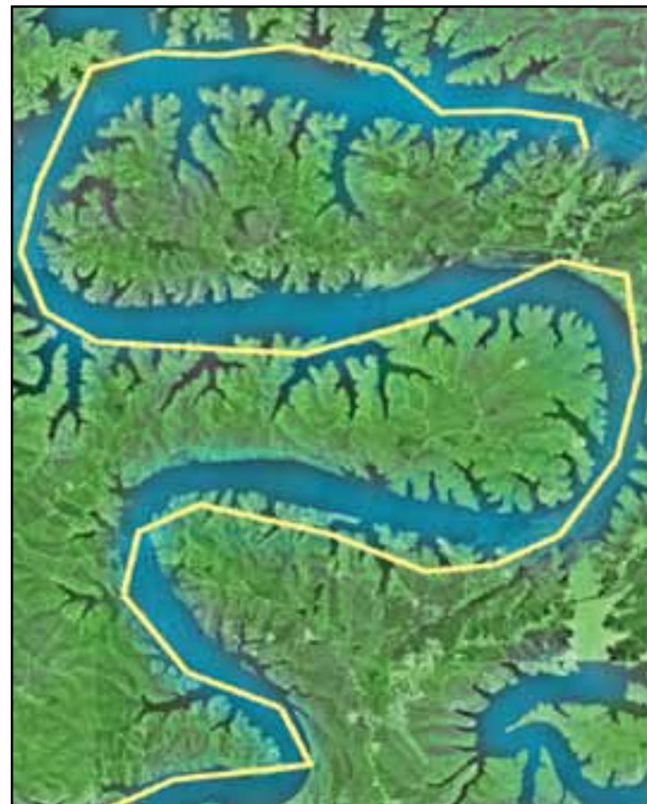
Pike's survey of the Osage River was remarkably accurate considering the primitive compass he used. The simple drawing in yellow represents his survey line of the river, as taken from his notes. The aerial photo underneath shows the same area today. Pike was only interested in following the main channel of the Osage and did not include the many tributaries.
