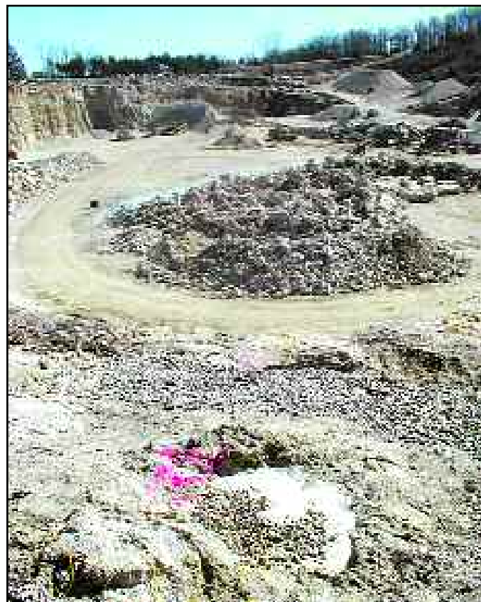
Holes drilled into the rock are filled with explosives and wired together prior to setting off 12,000 pounds of explosives.
