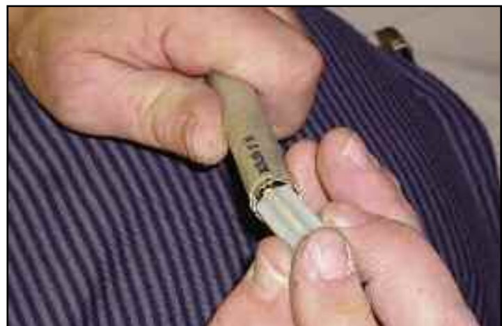
The assembled weight "package" is cemented into the shaft.
