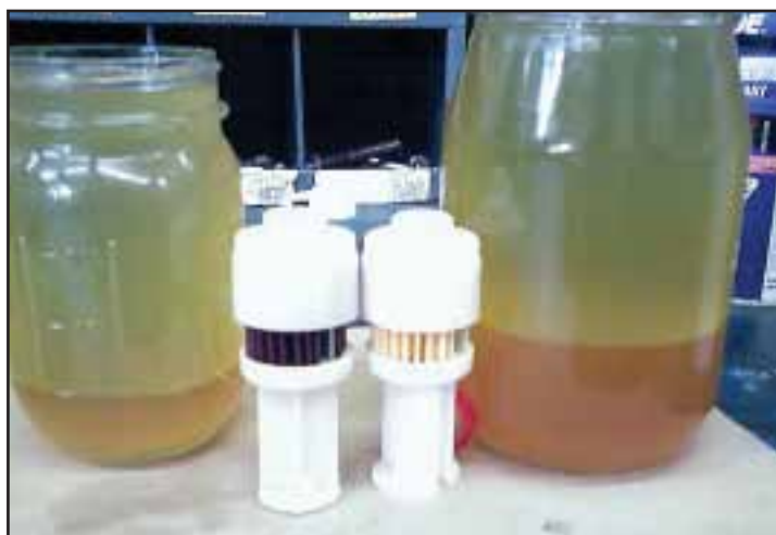
The phase separation of E10 fuel with gel at the bottom, with a clean fuel filter and a fuel filter blocked with the gel.
